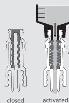
Straight through fluid path equal to an 18 g needle
