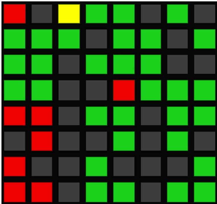
**USER INTERFACE** - The user interface is split in half. The top displays the sequencer grid. Active steps are green and inactive steps are not lit. The bottom displays selected Mode in red and the output voltage of the selected step in green. The current step marker is yellow. The cursor showing the selected step is a blinking red LED. The last step of the sequence is a solid red LED.
