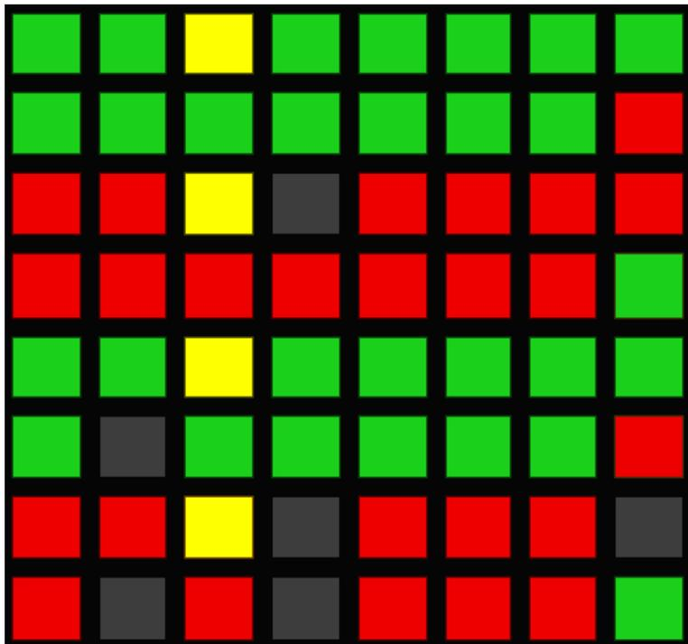
**USER INTERFACE** - The user interface is split into four sequencer grids. Active steps are green or red and inactive steps are not lit. The current step markers for each sequencer are yellow. The cursor showing the selected step is a blinking yellow LED. If the sequence is red, the last step is marked with a green LED. If the sequence is green, the last step of the sequence is marked with a red LED.
