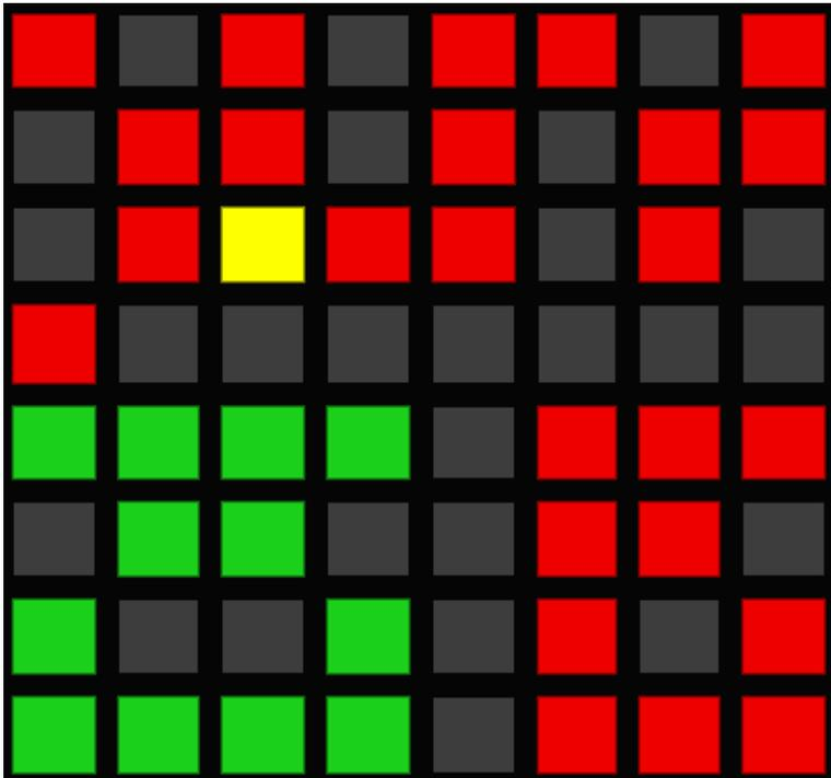
**USER INTERFACE** - The user interface is split in half. The top displays the sequencer grid. Active steps are red and inactive steps are not lit. The bottom displays the length of the sequence in green and the number of beats in red. The current step marker is yellow.
