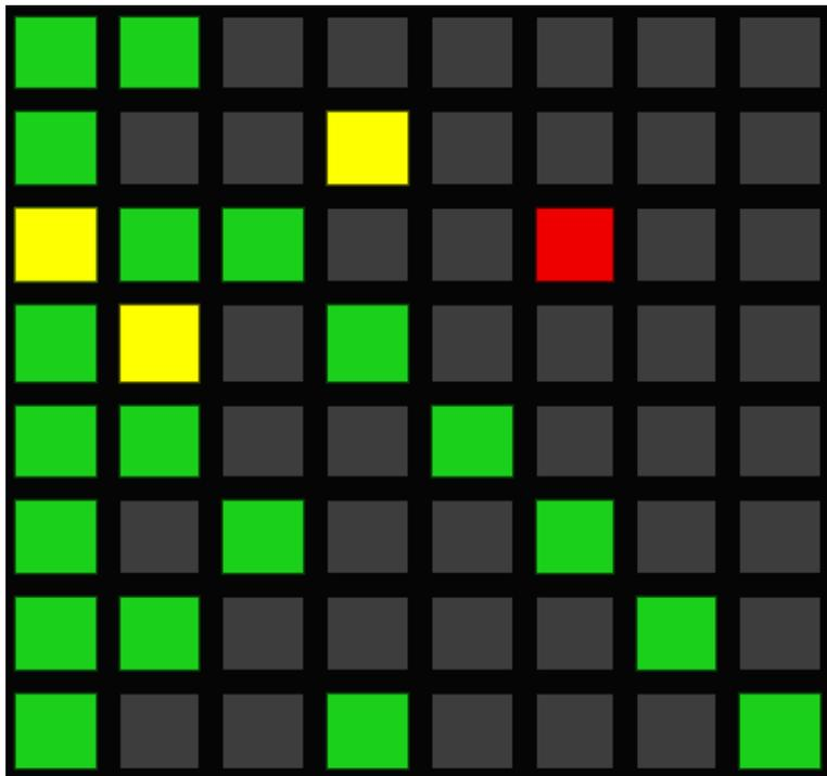
**USER INTERFACE** - Clock divisions are represented by green LEDs. The red LED represents the selected output. The Yellow LEDs represent the unselected outputs.
