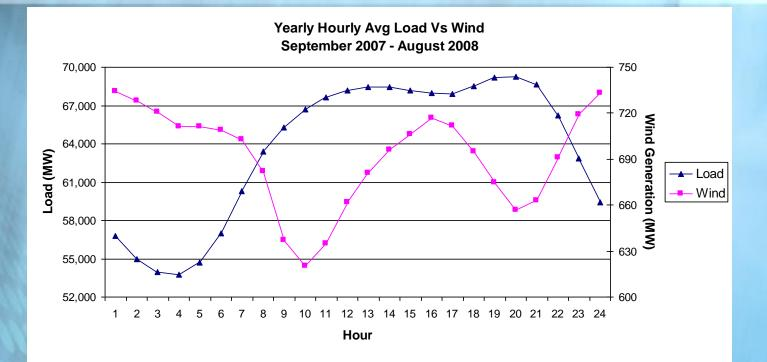
Additional on-line capacity needed to follow wind output and load
