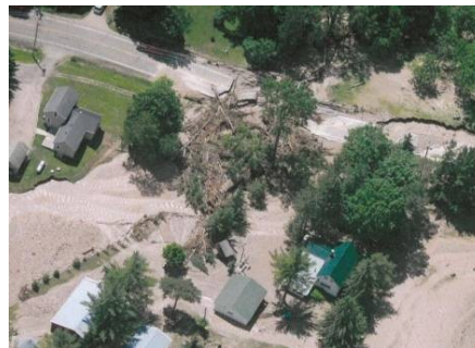
Below: State Highway 113 culvert debris jam
