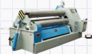
101-10-8 (1/2" x 8') hydraulic pinch pyramid plate bending machine.
