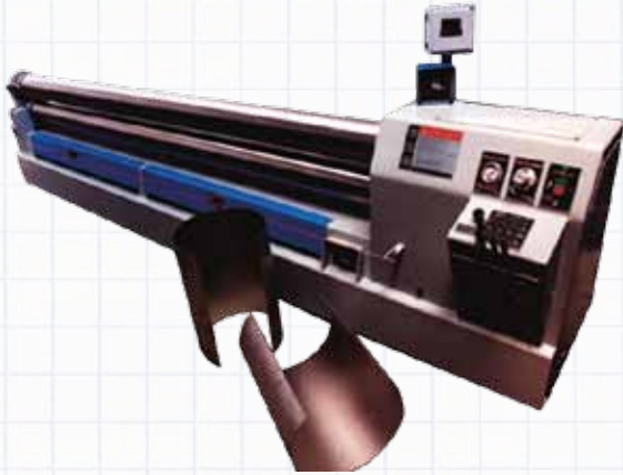
K-9-12 (.164" x 12') with standard dial pointer roll position indicator on bending roll. This machine is used to roll column covers.
