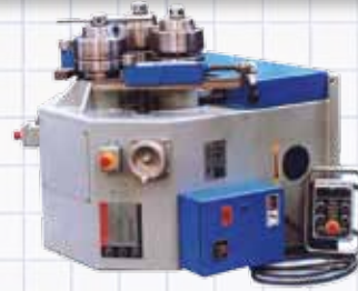
Model AR-31 (3 x 3 x 3/8 Capacity) angle roll with standard AR-520 control.
