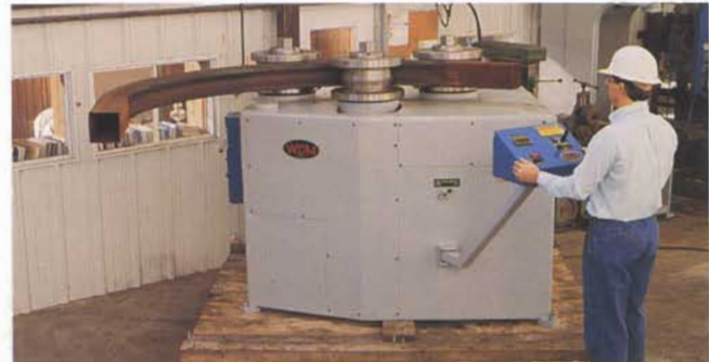
Special Rolls For Square & Rectangle Tubing
