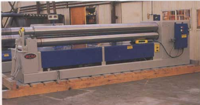
Hydraulic Initial Pinch Rolls
