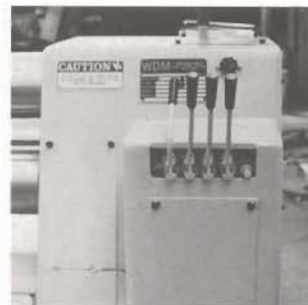
Manual Valve Type Control
