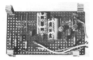
Anyways, I fitted a pair of probes to my plastic washer bottle using solder tags and wired the box inside along with the amber warning light. During testing I found that water sloshed around a lot and bridged the probes where they were fitted inside the bottle at the top: this gave a false reading of "bottle fullness". So I reduced the sensitivity of the circuit around TR1.
