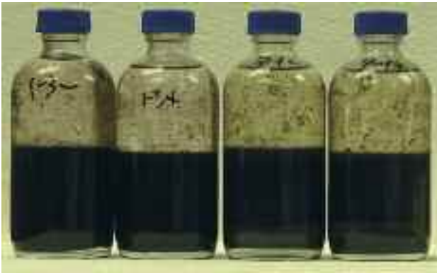
Fig.7. 125 ml hydrolysis/extraction bottles after hydrolysis, extraction, and centrifugation. The acid hydrolysate is dark material on bottom and the solvent extract of that hydrolysate is the clear liquid on top. This liquid was removed by suctioning and processed through the cleanup described in the materials and method section.
