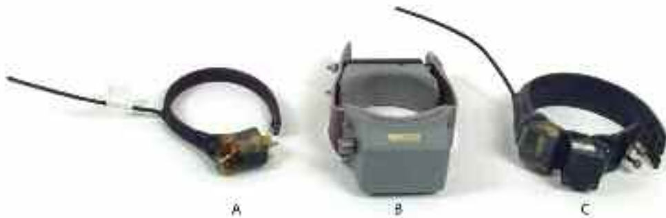
Fig.1. Collar types tested (A) VHF (B) VHF/GPS-GSM and (C) VHF with programmed drop off buckle.
