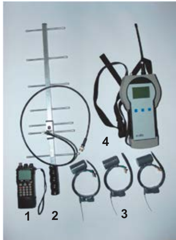
Fig.7. Tracking equipment: 1- VHF Receiver, 2-Yagi antenna, 3-radio collars, 4-base station for coordinate downloads.
