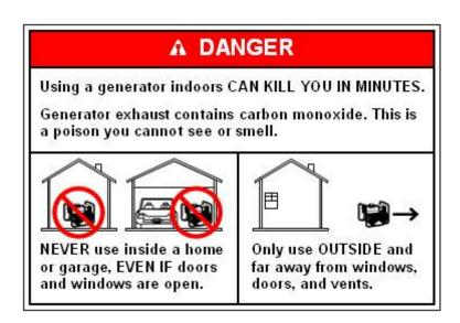
If you start to feel sick, dizzy, or weak while using a generator, get to fresh air **RIGHT AWAY. DO NOT DELAY**. The CO from generators can rapidly kill you.
