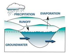
This means there is no inlet or outlet, so the lakes fill up through precipitation or runoff, supplemented by groundwater in the immediate drainage area. For this reason, the levels of both lakes fluctuate from season to season and year to year.
