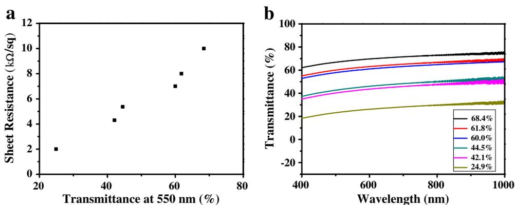
**Fig. 4.** (a) Sheet resistance versus optical transmittance at 550 nm for RGO film. (b) Optical transmittance of different RGO films on flexible glasses (the numbers showed in the box are the transmittances of RGO films at the wavelength of 550 nm).
