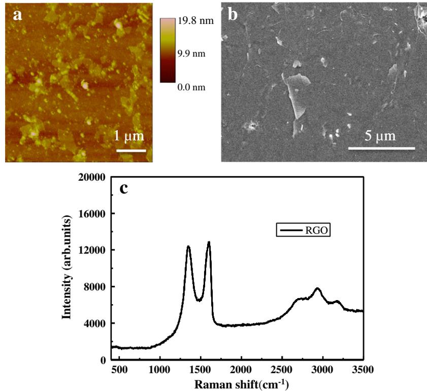
**Fig. 3.** (a) The AFM image of GO flakes. (b) The SEM image of a typical RGO flake deposited on flexible glass substrate. (c) Raman spectrum of RGO film excited with a laser wavelength of 514 nm.
