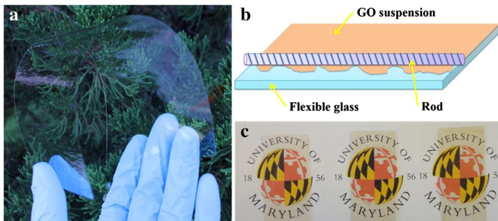
**Fig. 1.** (a) Flexibility of the transparent glass. (b) The schematic procedure of producing transparent and flexible GO coated glass by Meyer rod coating. (c) Uniform printing with GO ink on flexible glasses (transparency from left to right: 70%, 50%, and 30%).
