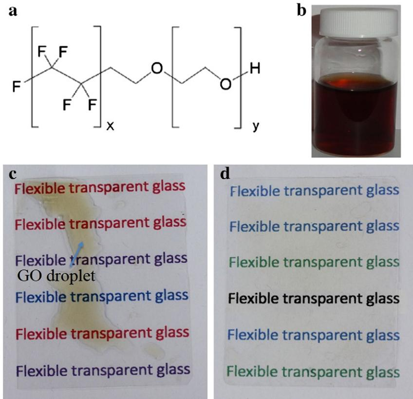
**Fig. 2.** (a) Molecular formula of the chosen Zynol surfactant. (b) Water-based graphene oxide ink containing Zynol surfactant. (c) Agglomeration occurs for an ink without Zynol additive. (d) Uniform coating of GO ink with Zynol on flexible glass.
