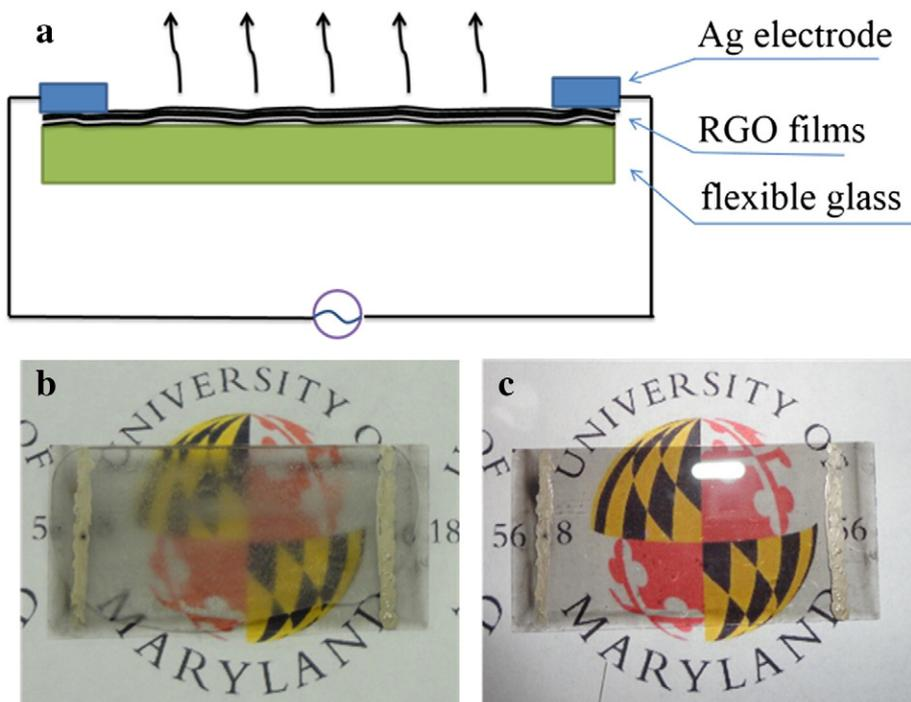
**Fig. 5.** (a) Schematic diagram of RGO films on flexible glass with an electrode pair. Defrosting results (b) before and (c) after annealing process of the RGO film with transparency 45% and sheet resistance  $5370 \Omega/\text{sq}$ .
