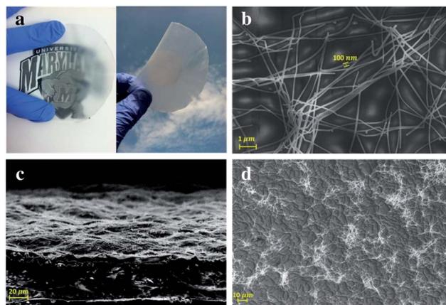
Fig. 2 (a) Optical image of Ag NW transparent paper; (b) SEM of Ag NW with diameter of 100 nm; (c) SEM of cross-section of Ag NW transparent paper; (d) top view of Ag NW transparent paper demonstrating embedded Ag NW network.
