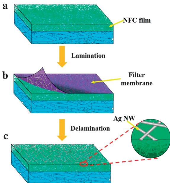
Fig. 1 Schematic of Ag NW network embedded in a nanopaper surface on the transparent paper. (a) Nanofibrillated cellulose was filtered through TEMPO-treated paper to form a smooth surface, (b) with a novel lamination process, a filtered Ag NW network is embedded in the smooth NFC surface, and (c) the final structure is a uniform Ag NW network embedded onto the surface of transparent paper.
