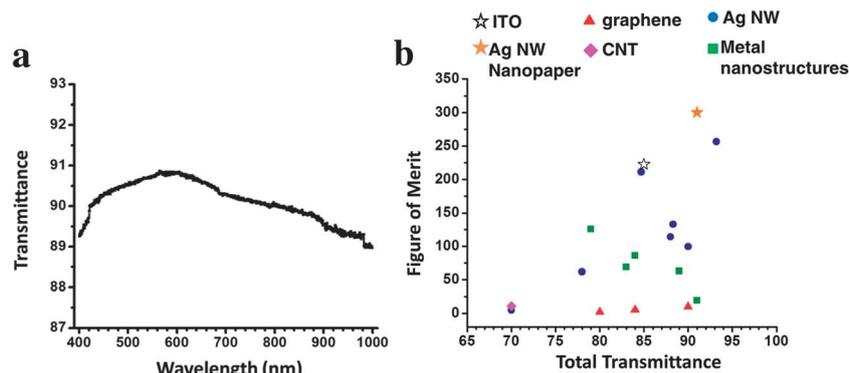
Fig. 3 (a) Total transmittance versus wavelength of Ag NW paper; (b) figure of merit versus total transmittance for previous TCE reports, ITO, and our Ag NW paper.<sup>15,17,29–35</sup>
