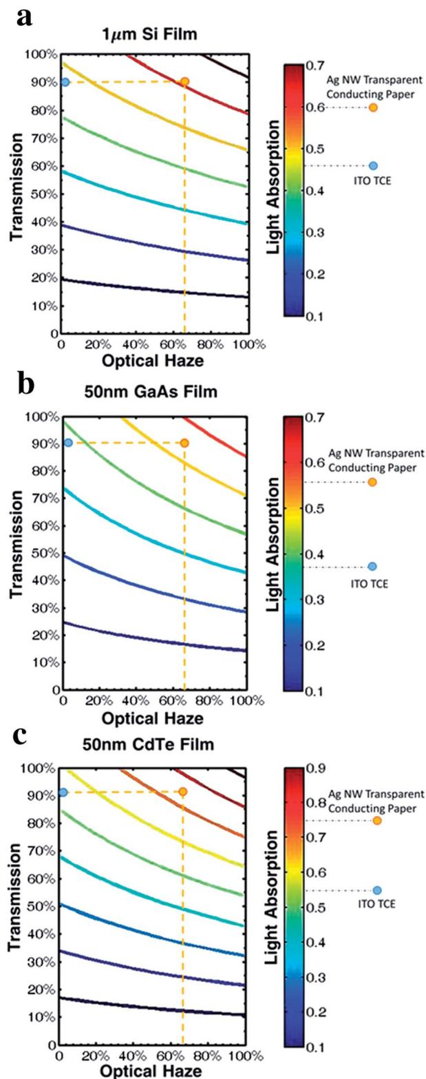
Fig. 5 Light absorption dependence of a structure including either a TCE with varying optical properties and an absorber layer (a) a  $1\ \mu\text{m}$  thick Si film, (b) a 50 nm thick GaAs film, and a 50 nm thick CdTe film. Light absorption in these absorbers for a highly transparent ITO TCE and our Ag NW paper TCE are compared as well.
