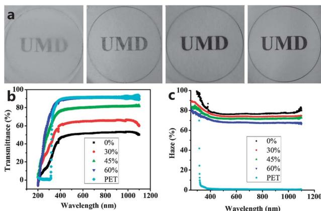
**Fig. 2** Optical properties of cellulosic paper at different weight ratios of NFC to whole paper. (a) The visual appearance of the cellulose paper. The weight ratio of NFC to paper from left to right is 0%, 30%, 45% and 60%. (b) Total light transmittance of the cellulose paper at various weight ratios of NFC. (c) The haze value vs. wavelength for transparent paper with different NFC ratios and PET.
