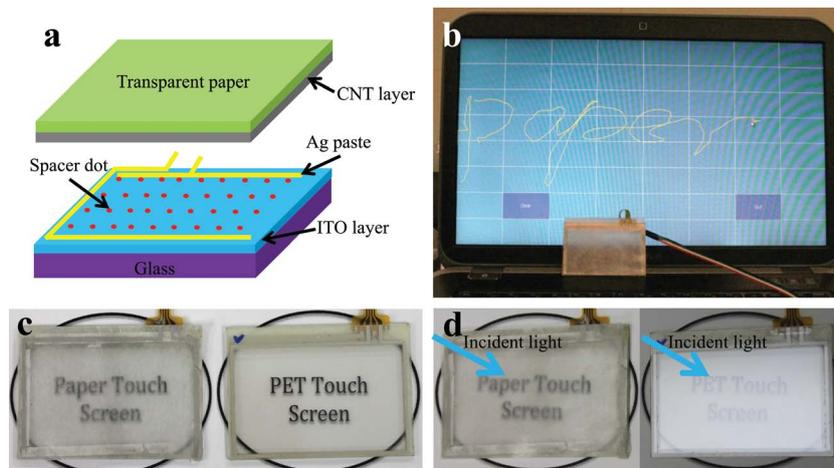
**Fig. 5** (a) A schematic structure of a transparent four-wire touch screen with nanostructured paper. (b) An assembled paper touch screen was used to simulate typical “paper” with the help of eGalaxTouch software from TVI Electronics LLC. (c) Left: a paper touch screen, right: a PET touch screen. (d) Two types of touch screen exposed to sunlight: a paper touch screen without glare (left) and a PET touch screen with great glare (right). All pictures were taken at a similar angle.
