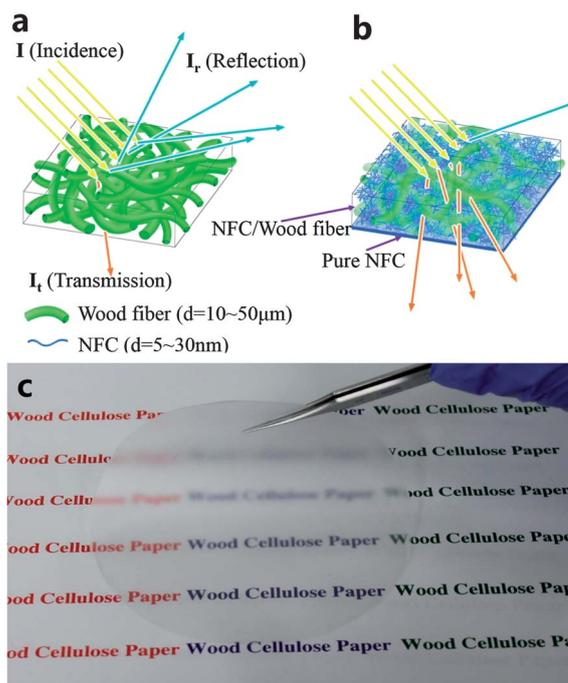
**Fig. 1** (a) Opaque cellulosic paper made of wood fibers. (b) Transparent hybrid paper consisting of two layers: the bottom layer is made of NFC and the top layer is produced by saturating NFC into the pores among the network of wood fibers. The widths of the wood fiber and NFC are 10–50  $\mu\text{m}$  and 5–30 nm, respectively. (c) Photo of the designed all-cellulose hybrid transparent paper with a thickness of 70  $\mu\text{m}$ .
