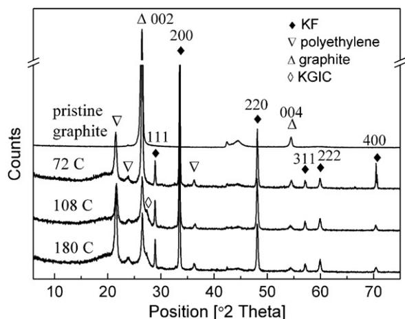
Fig. 6. X-ray diffraction patterns of resultant compounds after galvanostatic electrolysis in molten KF at 1163 K.
