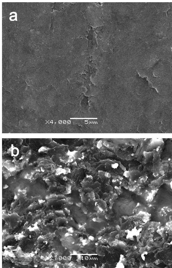
Fig. 7. SEM photographs of graphite electrodes surface: (a) before electrolysis; (b) after electrolysis—note that the electrode was washed with distilled water to get rid of the solidified electrolyte on surface.
