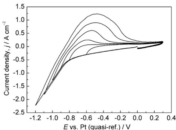
**Fig. 3.** A series of cyclic voltammograms recorded on graphite electrode with various cathodic switch potentials in molten KF at 1163 K. Potential scan rate =  $100 \text{ mV s}^{-1}$ .
