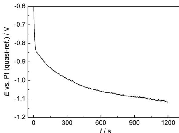
Fig. 5. Chronopotentiogram of graphite electrode in molten KF during cathodic polarization with at 1163 K. Step current = 200 mA.
