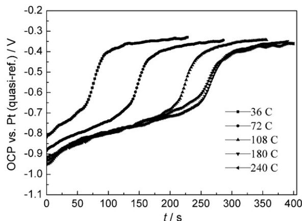
**Fig. 4.** OCP variations of the graphite electrodes after galvanostatic electrolysis in molten KF at 1163 K. The inserted numbers behind the legends denote the transferred electricity during galvanostatic electrolysis.
