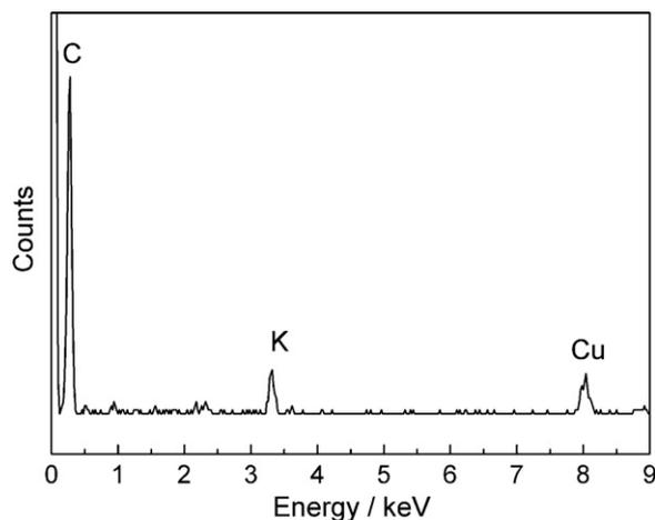
**Fig. 9.** Typical EDX spectrum of the sample shown in Fig. 8. The Cu and K profiles were built up from a TEM copper grid and the not completely removed electrolyte respectively.
