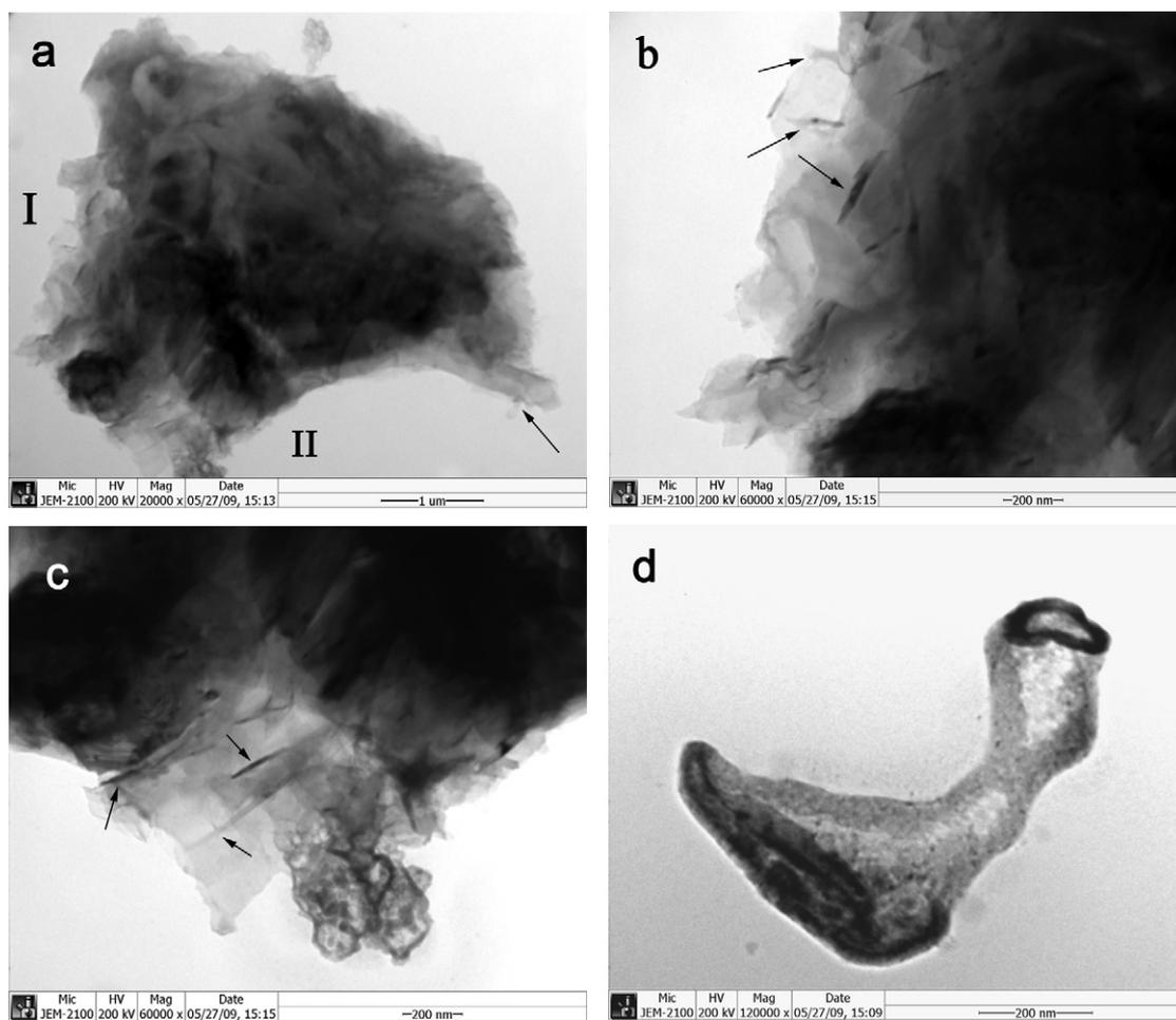
**Fig. 8.** TEM images of: (a) a representative sample obtained at the upper layer of the melts; (b) magnified image of local region I marked in photograph (a); (c) magnified image of local region II marked in photograph (a); (d) an individual dumbbell-like tube. The arrow marked in image (a) points to a tube. The arrows marked in image (b) and (c) point to the enrolled edges of thin sheets.
