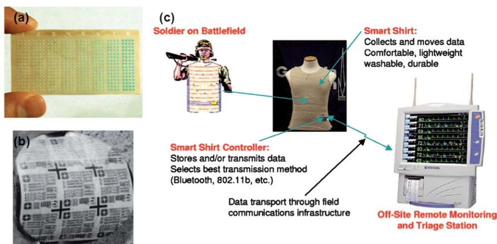
**Fig. 1** (a) A photograph of a paper-based 3D microfluidic device. (b) A photograph of pentacene TFTs and integrated circuits on paper. (c) The smart shirt in the field.<sup>3,13</sup>
