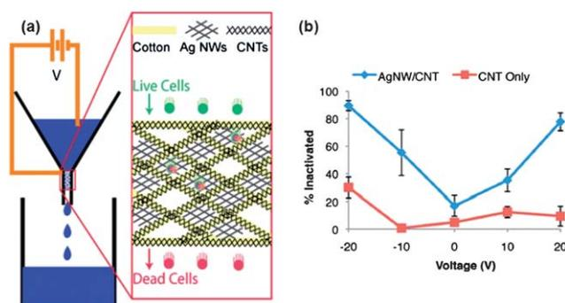
**Fig. 15** (a) Schematic of water filtration setup based on conductive cotton. A voltage is applied between the conductive textile and copper wire as water is filtering through the conductive textile. (b) Inactivation efficiency at different biases for AgNW/SWNT cotton as well as SWNT-only cotton.<sup>53</sup>
