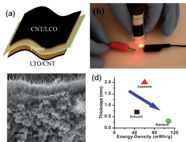
**Fig. 9** Integrated thin, flexible Li-ion paper battery. (a) Schematic of the final paper Li-ion battery device structure. The paper is used as both the separator and the mechanical support. (b) Picture of a highly flexible Li-ion battery lighting up a LED device. (c) SEM image of the cross section of SWNT/LTO double layer. (d) Comparison of our paper Li-ion battery with other flexible energy storage devices.<sup>45</sup>
