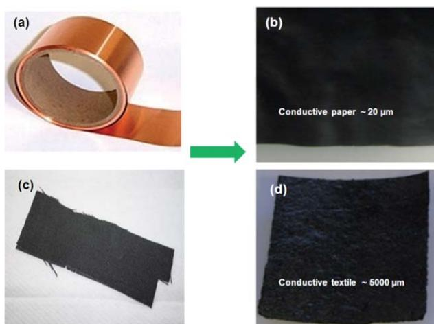
**Fig. 6** Shift from traditional conductors to new conductors based on paper and textiles. For thin conductors, conductive paper (b) replaces heavy metal foil, *i.e.* Cu foil (a). For 3D porous conductors, conductive textile (d) replaces carbon cloth (c).
