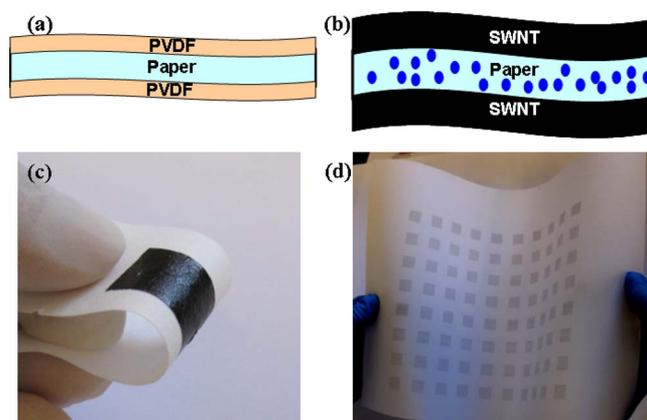
FIG. 1. (Color online) (a) Schematic of Xerox brand printer paper treatment with PVDF; this treatment is used to block the micron-sized pores to avoid short circuiting because of SWNT penetration. (b) Paper supercapacitor structure with SWNT film printed on both sides of the treated Xerox paper. The SWNT film is either Meyer rod-coated or ink-jet printed. (c) A photo of a Meyer rod-coated supercapacitor on Xerox paper. (d) A photo of ink-jet printed supercapacitor on Xerox paper.
