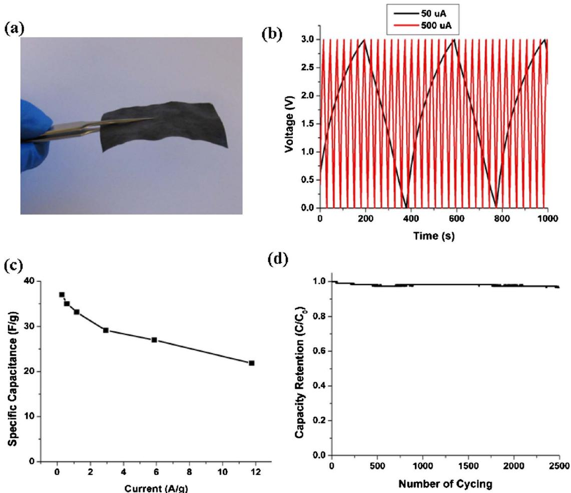
FIG. 3. (Color online) (a) A printed supercapacitor on a 30  $\mu\text{m}$  thick newspaper substrate/separator membrane. (b) Charge-discharge performance of a printed paper supercapacitor with paper as both separator and substrate. (c) Specific capacitance at different current density. (d) Cycling performance of a printed paper supercapacitor with 1  $\text{mA}/\text{cm}^2$  current.
