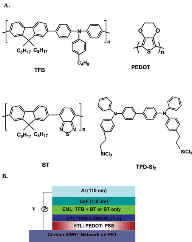
**Figure 2.** (A) Chemical structures of poly(9,9-dioctylfluorene-*co*-*N*-(4-butylphenyl)diphenylamine) (TFB), poly(9,9-dioctylfluorene-*co*-benzothiadiazole) (BT), poly(3,4-ethylenedioxythiophene) (PEDOT), and 4,4'-bis[*p*-trichlorosilylpropylphenyl]phenylamino-biphenyl (TPD-Si<sub>2</sub>). (B) Structure of a PLED device having a carbon SWNT film anode.
