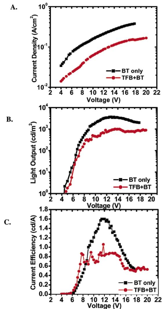
**Figure 5.** Response characteristics of PLEDs having the structures: (Device 3) SWNT(30 nm)/TFB + TPDSi<sub>2</sub>(25 nm)/TFB + BT(70 nm)/CsF(1.8 nm)/Al(110 nm) and SWNT(30 nm)/TFB + TPDSi<sub>2</sub>(25 nm)/BT(70 nm)/CsF(1.8 nm)/Al(110 nm). Key: (A) current density vs voltage; (B) luminance vs voltage; (C) current efficiency vs voltage.
