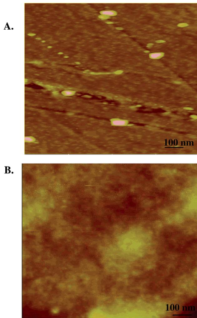
**Figure 3.** (A) AFM image of SWNT film with a spin-coated PEDOT-PSS overlayer. The rms roughness is 4 nm from the AFM image. (B) AFM image of SWNT film with a spin-coated PEDOT-PSS:MeOH (1:2) overlayer. The rms roughness is 0.96 nm from the AFM image.
