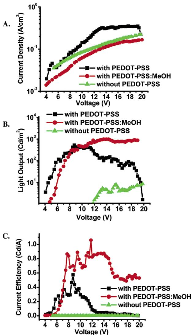
**Figure 4.** Response characteristics of PLEDs having the structures: (device 1) SWNT(30 nm)/PEDOT-PSS:MeOH(30 nm)/TFB + TPDSi<sub>2</sub>(25 nm)/TFB + BT(70 nm)/CsF(1.8 nm)/Al(110 nm), (device 2) SWNT(30 nm)/PEDOT-PSS(30 nm)/TFB + TPDSi<sub>2</sub>(25 nm)/TFB + BT(70 nm)/CsF(1.8 nm)/Al(110 nm), and (device 3) SWNT(30 nm)/TFB + TPDSi<sub>2</sub>(25 nm)/TFB + BT(70 nm)/CsF(1.8 nm)/Al(110 nm). Key: (A) current density vs voltage; (B) luminance vs voltage; (C) current efficiency vs voltage.
