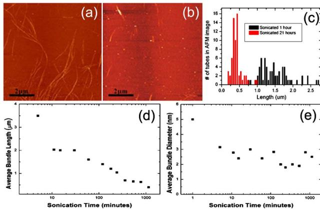
FIG. 1. (Color online) Effects of sonication on SWNT bundle length and diameter. [(a) and (b)] AFM image of SWNTs absorbed on a silicon wafer after (a) 1 h and (b) 21 h of sonication time. (c) Histogram of bundle length distribution taken from several AFM images for 1 h (black) and 21 h (red) of sonication. Plot of the (d) average bundle length and (e) average bundle diameter for various sonication times measured from AFM images.
