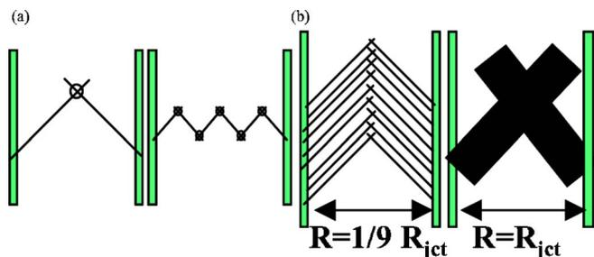
FIG. 3. (Color online) Qualitative argument for the dependence of the dc conductivity of SWNT networks on the average bundle length and diameter. (a) Longer tubes lead to fewer junctions to cross the surface, which leads to higher conductivity. NT-NT junctions are circled. (b) Larger bundles lead to lower conductivity as  $\sigma \sim D_{av}^{-2}$  for stiff bundles where  $R_{jct}$  is independent of the bundle diameter.
