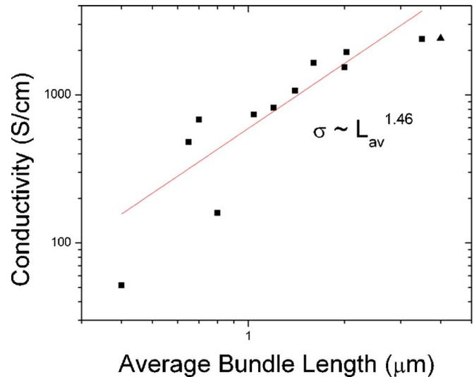
FIG. 2. (Color online) DC conductivity of SWNT networks vs average bundle length in the network. Data are fit to a power law,  $\sigma_{dc} \sim L_{av}^{\alpha}$  with  $\alpha = 1.46$ . Data for 4  $\mu\text{m}$  length tube (triangle) is excluded from the fit because of the larger bundle diameter for that data point.
