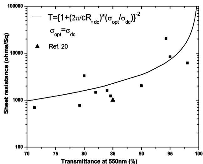
**Figure 3.** Transmittance at 550 nm for NTN of various sheet resistances. The solid line is a fit to eq 3. We find that  $\sigma_{ac} = \sigma_{dc}$  provides the best fit for the NTN data. Our data are in agreement with data provided by Manohar et al.
