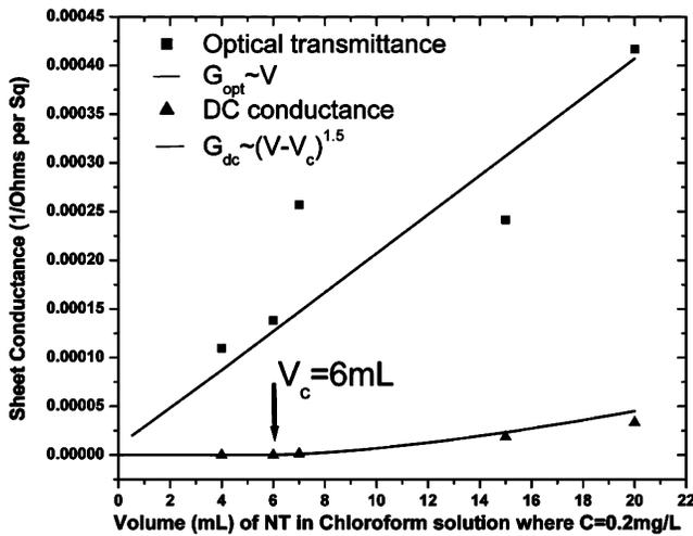
**Figure 4.** DC and optical sheet conductance at 800 nm vs volume of NT solution. The optical conductance was calculated using eq 3 from the measured transmitted power at 800 nm. The arrow indicates the DC percolation threshold. The optical conductance is proportional to nanotube density.
