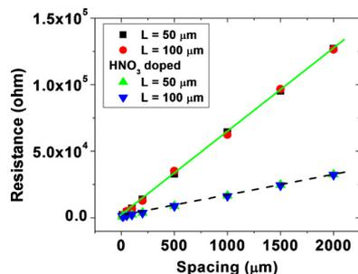
FIG. 3. (Color online) Influence of the doping process on the contact resistance. The resistance was measured by 2-point method for doped and undoped SWCNT films with Pt leads.
