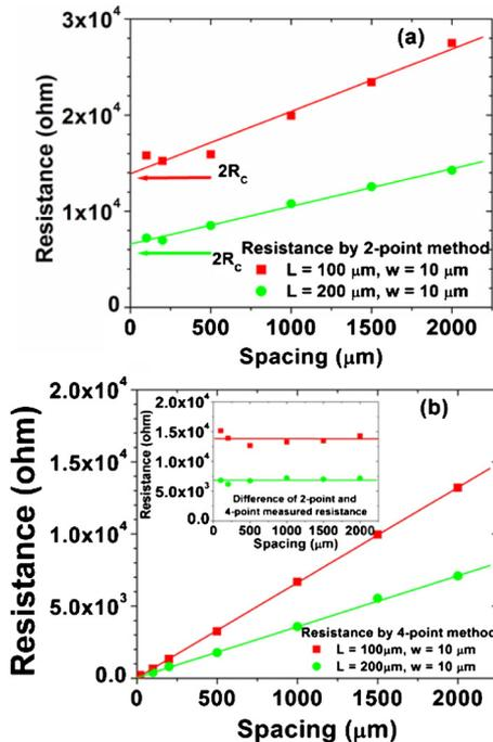
FIG. 2. (Color online) Measured resistance at different spacings for copper leads. (a) 2-point resistance as a function of lead spacing. Contact resistance  $R_c$  is determined from intersect with y-axis. (b) Resistance measured by 4-point method vs lead spacing. The inset shows the difference,  $2R_c$ , of 2-point and 4-point resistances.
