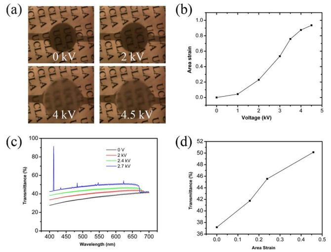
FIG. 2. (Color online) (a) Isotropically stretched CNT films under different applied voltages showing the increase in strain. (b) Area strain as a function of applied voltage, as shown in (a). (c) Spectra of stretched CNT films in visible range. As the CNT film was stretched, the transmittance increased due to the thinning of the nanotube film. (d) Transmittance at 550 nm as a function of area strain.
