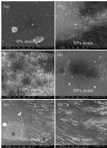
FIG. 3. (a) SEM of sprayed CNT film on 3M VHB 4905 substrate. (b) SEM of CNT film under 50% strain. (c) SEM of CNT film under 150% strain. (d) Enlarged view of the CNT film under 50% strain to show the cracks built up during stretching. (e) Enlarged view of the CNT film under 50% strain to show the boundary between high conductive area and low conductive area separation. (f) Enlarged view of the CNT film under 50% strain.
