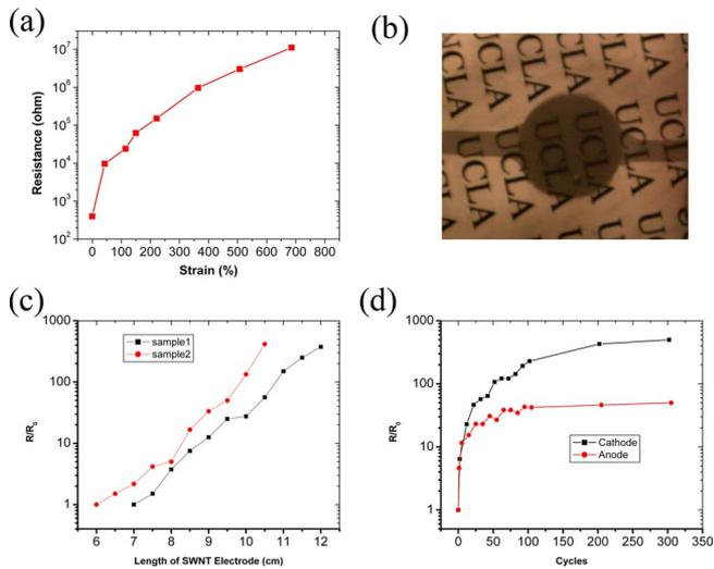
FIG. 1. (Color online) (a) Resistance as a function of strain under unidirectional stretching. (b) Set up for isotropically stretching of CNT thin film with layered structures. The circular area is where the cathode and anode CNT films overlap. (c) Resistance change as a function of strain for isotropically stretched CNT films in setup (b). (d) CNT film resistance change after cyclically actuating the films between 0% and 100% strain multiple times.
