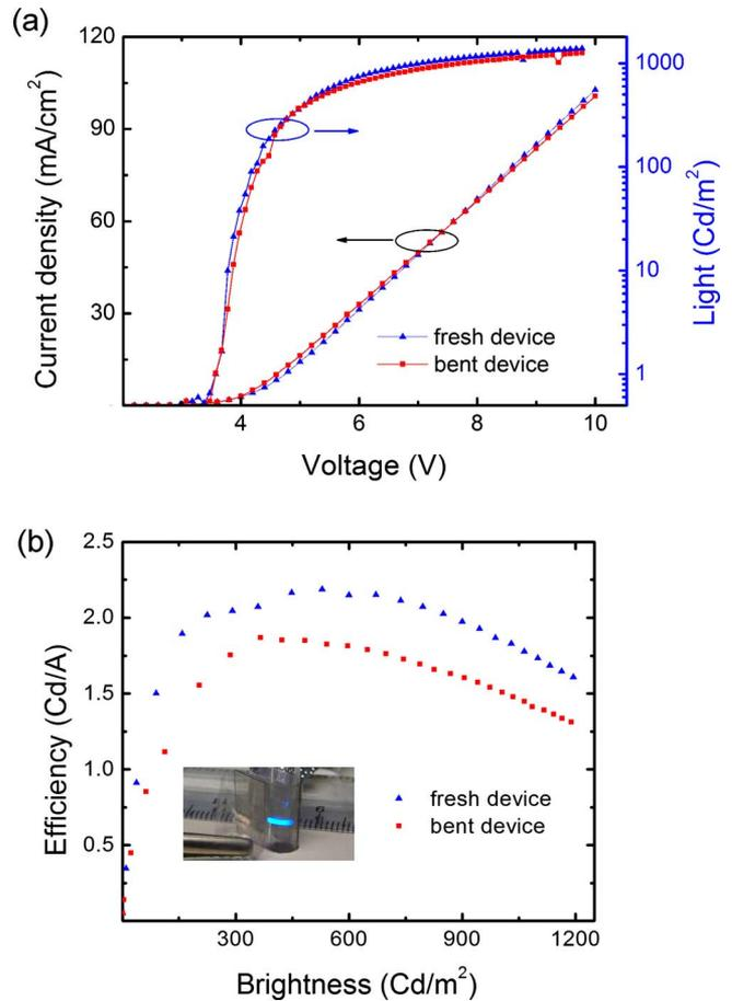
FIG. 3. (Color online) (a) Current and light emission intensity of the blue emission device at flat state before and after being bent to a 2.5 mm radius. (b) Efficiency of the flat device before and after being bent to a 2.5 mm radius (inset shows an emission photo at 6 V of the blue emission device wrapped around a 5 mm diameter glass tube).
