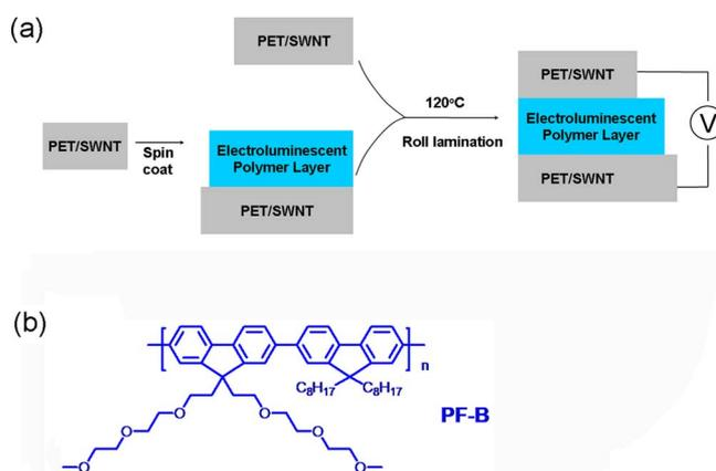
FIG. 1. (Color online) (a) Illustration of the lamination process to fabricate a polymer light emitting device and (b) Chemical structure of the blue (PF-B) emitting polymer.
