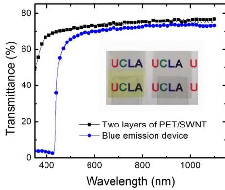
FIG. 2. (Color online) Optical transmittance spectra for two layers of SWNT/PET laminate and blue emission light emitting device. Inset shows a photograph of two layers of SWNT/PET laminate and different color light emitting devices placed on top of a sheet with color printed "UCLA" patterns.
