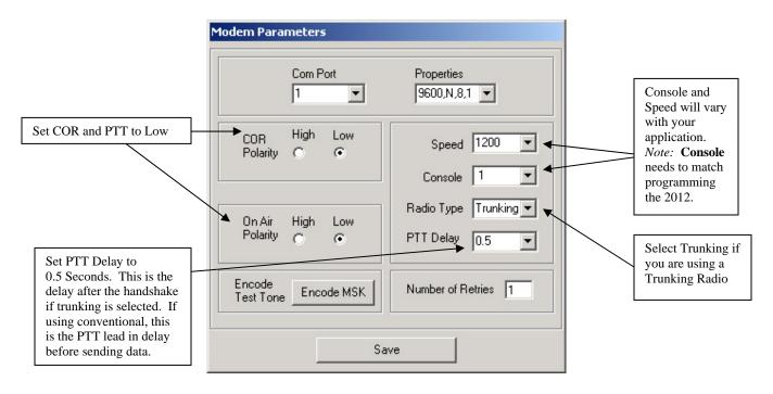
The figures below shows how a typical RasTrac I/O processor will be set up when connected to a 2016 and M1225 radio. To access the I/O configuration, select the *Edit* pull down menu from the RasTrac I/O Processor. From the *Input/Output Configuration* screen, select the *Protocol* to be **PYRAMID**. Then click *Properties* to configure the 2016.
