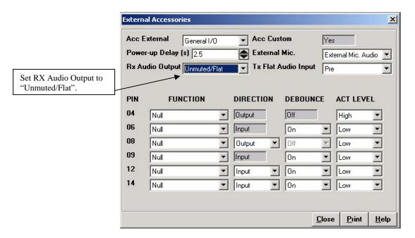
Set the *Rx Audio Output* to "Unmuted/Flat". This will enable all RX audio from the discriminator of the radio to be available on the accessory connector of the radio.
