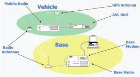
modem simply transmits the data over the voice channel all other bus drivers can hear the short data burst each time any GPS update is sent.
