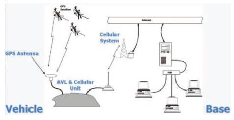
The network then routes the data to an Internet Protocol (IP) address to be picked up by the mapping software.
