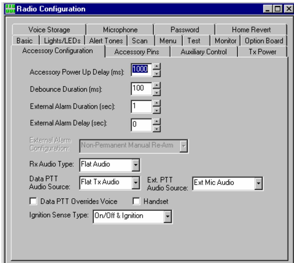
1. Set the **Rx Audio Output** to “**Flat Audio**”. This will enable all RX audio from the discriminator of the radio to be available on the accessory connector of the radio.
