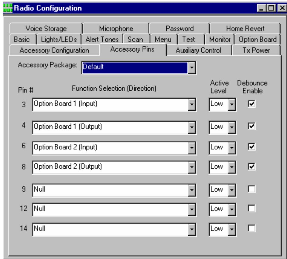
1. Program **Pin 3** of the accessory connector for “**Option Board 1 (Input)**” **Active Low**
