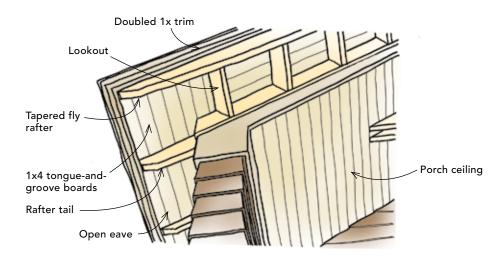
eave. This design increases the sheltering effect by extending the ceiling beyond the wall planes. It also provides ample shade and sheds water far from the face of the siding.
