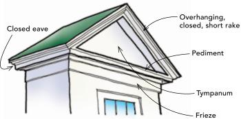
interpretations. A short, closed rake is typically supported by blocking. If a less-ornate treatment is called for, replace the contoured molding that extends around the eaves and up the rake with layered flat trim.
