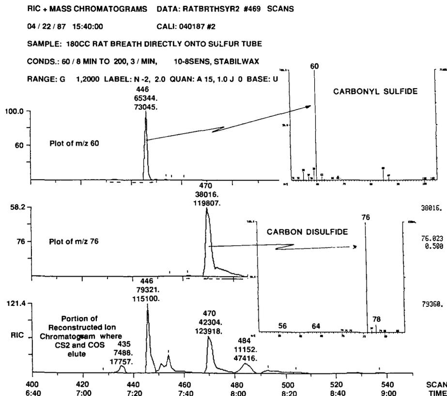
FIG. 1. Reconstructed ion chromatograms of rat breath showing molecular ions for COS and CS<sub>2</sub>. The spectrum of CS<sub>2</sub> consists mainly of the molecular ion m/z 76, the sulfur-containing isotope ion at m/z 78 as well as a small fragment ion at m/z 64. The spectrum of COS consists primarily of its molecular ion at m/z 60, and an isotope ion at m/z 62.
