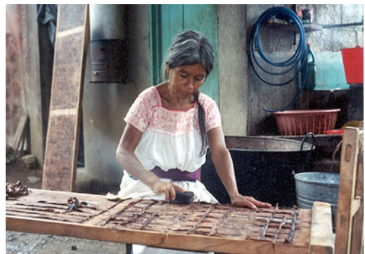
Fig. 2. Bark paper manufacturing. Stone beaters have been used since the pre-Hispanic period to pound bark fibers and form the bark sheets.
