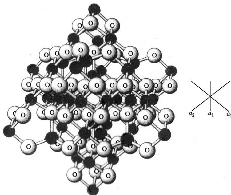
**Figure 6** Magnetite. The crystal structure of magnetite, a member of the spinel group of minerals. The  $[111]$  crystallographic direction is vertical to show the horizontal appearance of cubic-close-packed oxygen (O) atoms.  $\text{Fe}^{2+}$  and  $\text{Fe}^{3+}$  are in tetrahedral and in octahedral interstices (both dark colored) (after Gaines *et al.*, 1997, p. 293).
