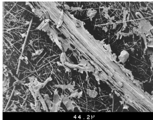
Figure 2. SEM image of isolated bamboo mineral material. The bamboo mineral has been mounted on glass filter with fibres of approximately 1\ \mu\text{m} in diameter: the filter appears as the threaded matrix of the image. The bar represents 44.2 \mu\text{m} .
