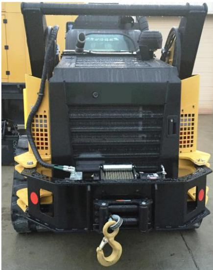
Supertrak is proud to offer an Industry Leading Hydraulic Winch Kit for your Caterpillar® C, D-Series Models. A Hydraulic Winch Kit will provide 15,000 or 20,000 lbs of pull when ground conditions are at the worst in applications like Forestry, Recycling for recovery efforts.
