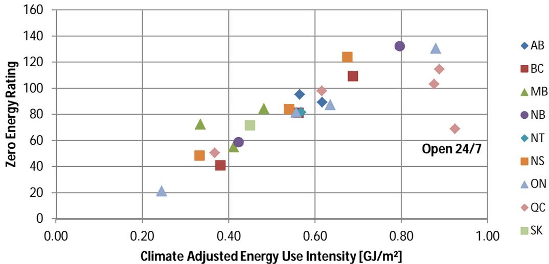
Figure 7: Zero Energy Rating versus Climate Adjusted Energy Use Intensity – Medium Offices
