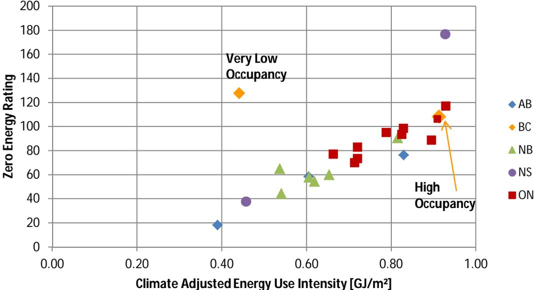
**Figure 10: Zero Energy Rating (MNECB 1997 Reference) versus Climate Adjusted Energy Use Intensity – Primary Schools**
