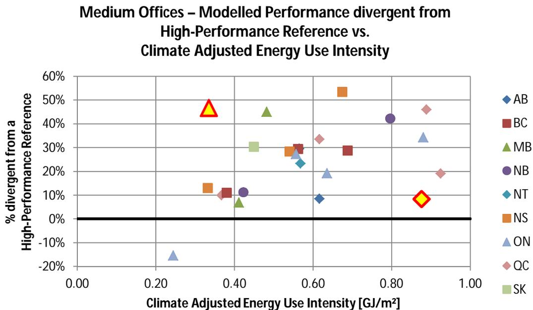
Figure 5: Performance related to a High-Performance Reference versus Climate Adjusted Energy Use Intensity – Medium Offices
