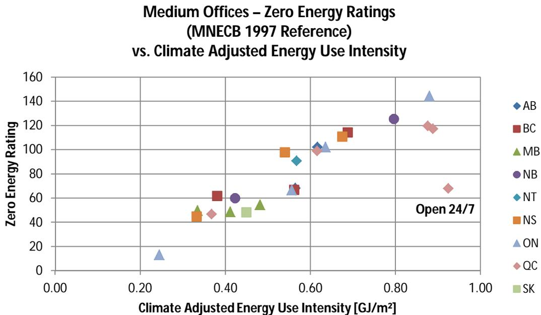
Figure 9: Zero Energy Rating (MNECB 1997 Reference) versus Climate Adjusted Energy Use Intensity – Medium Offices
