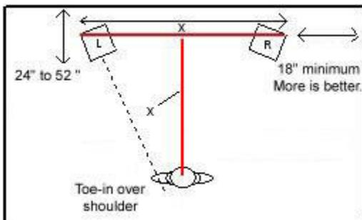
We developed the 'Equal-Legged T' from years of experiments in rooms from 10- to 100' wide. Since visual acuity for the fixed eye "falls off" at the 53-degree span, we believe a link exists between the point at which our peripheral vision "falls off" and our keenest sense of hearing begins. This layout will allow images to develop outside of the speakers' boundaries, if such information is in the recording.
