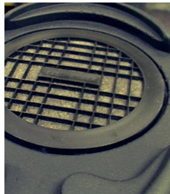
A resistive vent loads the rear of both Calypso and Pico Executive midrange cones, suppressing each one's natural low-frequency resonance. The Calypso's midrange enclosure adds a second-stage muffler over the rear of this vent.
