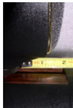
**3.** The helper will then add 3" (7.5cm) to the woofer distance and locate this new number on the tape while you hold the hook-end to the tweeter's grille and slide the tweeter to match this new number.
