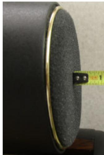
**4.** With the hook-end of the tape against the thumb-nut, measure and note the amount of Cocobolo trim exposed in front of it. Set the other tweeter to match this number.
