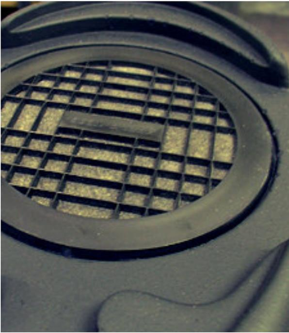
passing through the vent. Think of it as a second-stage muffler, for that is exactly what it is. It does not restrict the air flow through that vent.
