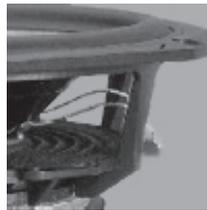
is required to stroke, as the math showed it would do. The voice coil driving the cone would be vented for cooling and releasing air pressures behind it which would otherwise inhibit motion.
