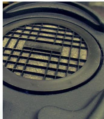
A resistive vent loads the rear of both Calypso HD and Pico Executive HD midrange cones, suppressing each one's natural low-frequency resonance. The Calypso HD's midrange enclosure adds a second-stage muffler over the rear of this vent.
