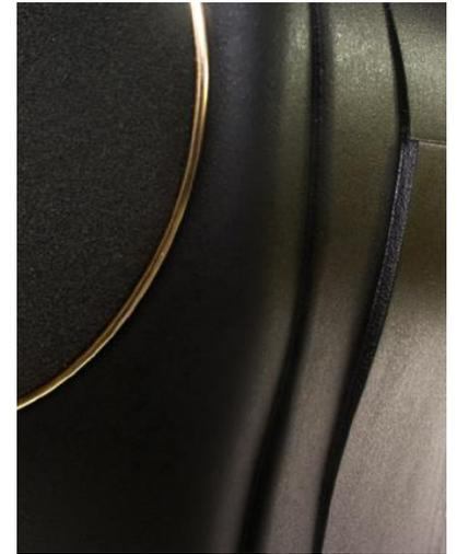
For this, Eos' tweeter has a **new absorptive material design** around it, which captures all the highs usually sent to its sides, and up and down as well. The channels between the discs present even more surface area for more sound absorption. The non-symmetric placement of the discs results in a more uniform sound absorption. Simple, economic, and completely effective!
