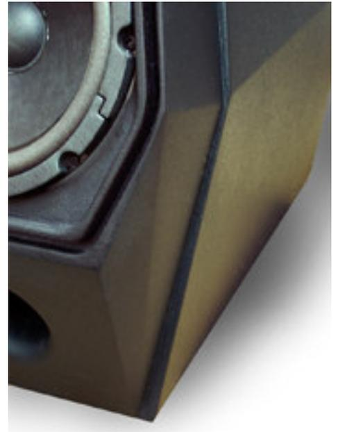
This woofer has a patented neodymium magnetic structure creating a powerful and uniform field around what is called an underhung voice coil. This large field always surrounds the woofer's voice coil, no matter how hard the coil is made to stroke, for complete control at all times. A highly flexible suspension allows proper motion of the cone on both very small signals and very large ones.
