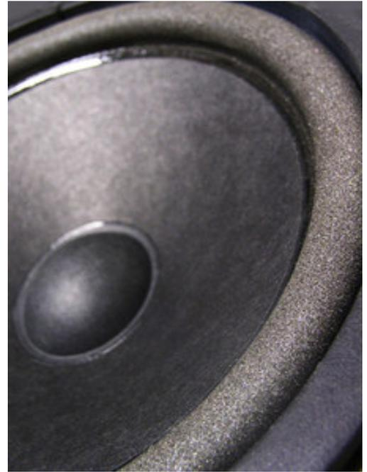
The chassis of this woofer is a rather light-gauge sheet metal, because the woofer's neodymium-magnet structure weighs just 10 percent of a regular magnet. However, we strengthen and deaden this chassis with a fiber-reinforced epoxy putty, as for Eos and Eos HD. The woofer is held in by eight screws, clamping its rim evenly and firmly to more than an inch of our solid Q-Stone™ marble.
