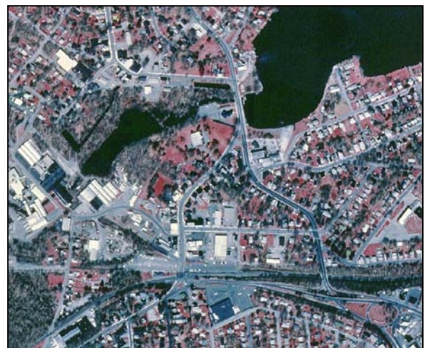
Digital orthoquad images (1m resolution) can be utilized to assess tree canopy.
