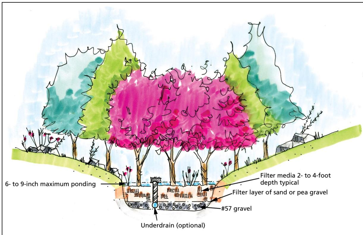
Figure 1. Bioretention and bioinfiltration facilities remove pollutants from storm water runoff using a filter medium.
