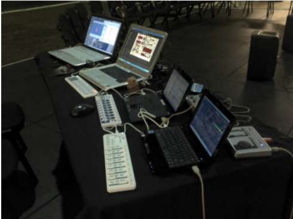
Figure 7: Computer setup by Warren Burt for Catherine Schieve's "Experience of Marfa." Astra Concerts, Melbourne June 1-2, 2013. Two laptops and two netbooks controlled by Korg control boxes.
