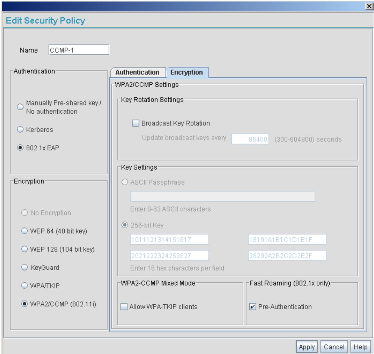
Preauthentication was designed for use by autonomous APs but works equally well between WLAN controllers to solve the same problem. Notice in figure 7 that Preauthentication is available in some controllers for the purpose of fast/secure roaming between controllers.
