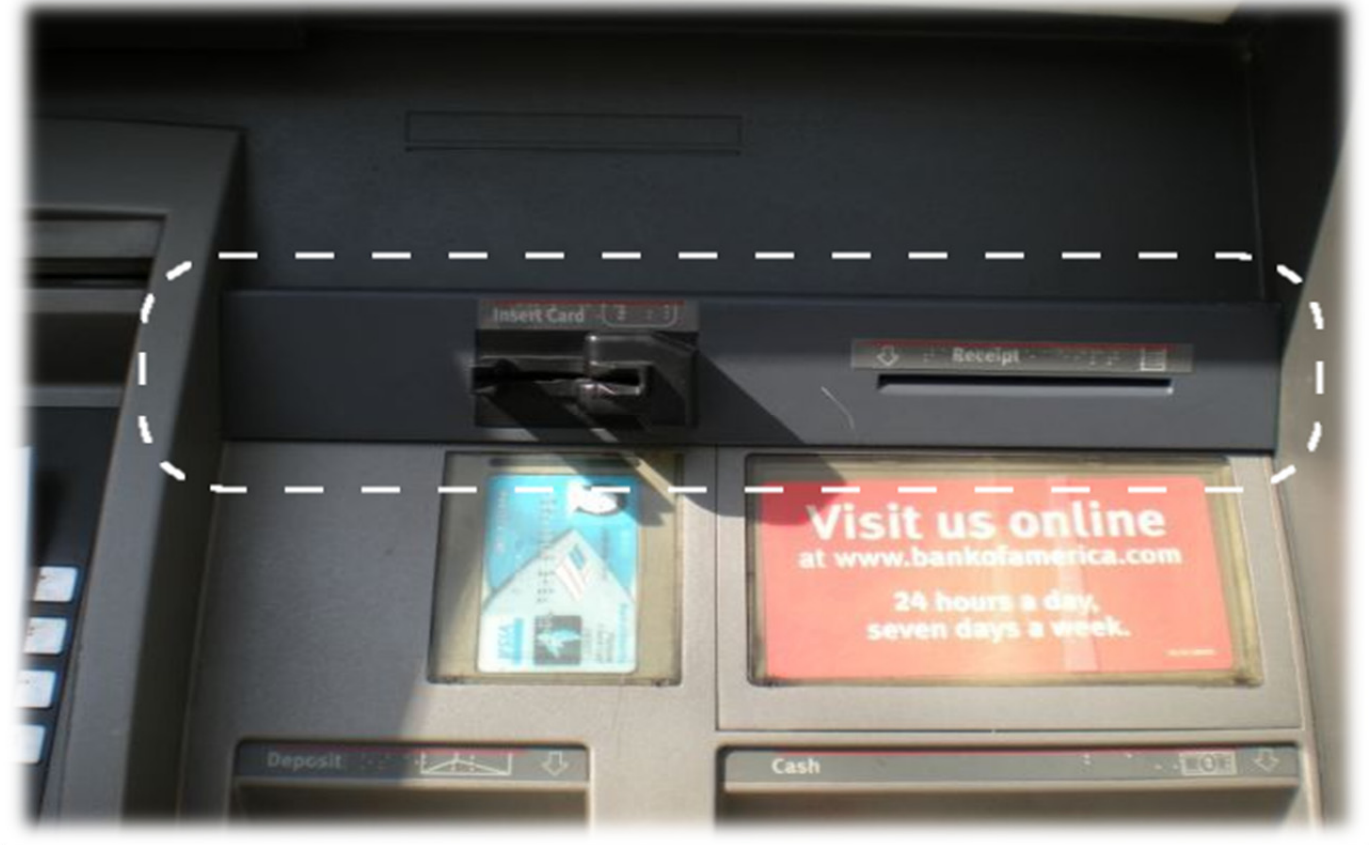
Figure 11: Skimmer on ATM Machine [19]
