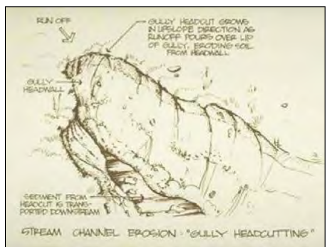
Figure 10-14. Gully erosion is complex; involving multiple failure processes.
