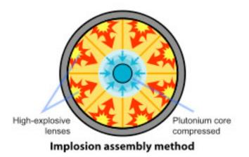
Such an implosion device is by no means simple; it requires painstaking engineering and careful testing. The Nagasaki bomb was made in this fashion. It was tested months ahead of time at Alamogordo, New Mexico.
