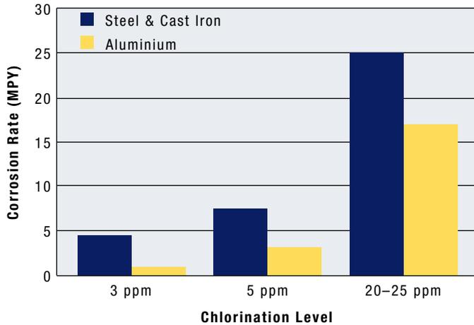
**Figure 7:** Carbon steel, cast iron, aluminum and stainless steel alloys were tested at three different chlorination levels and the average rate of metal loss determined in mils per year (mpy). The general corrosion rate of type 304 and 316 stainless steel was so low (<0.1 mpy) at all chlorination levels that it could not be graphed.
