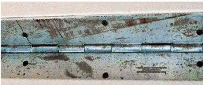
**Figure 5:** Carbon steel brushes were used by a cleaning contractor on this stainless steel door hinge that was installed beside an indoor swimming pool. The areas with carbon steel contamination are rusting. Photo courtesy of TMR Consulting
