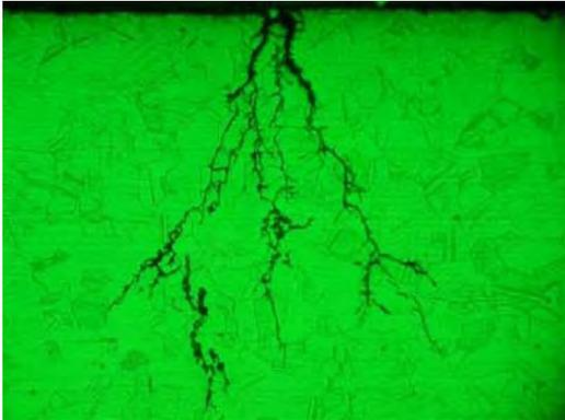
**Figure 13:** This magnified cross-section of a sample from the roof deck illustrates the extensive SCC that occurred.
