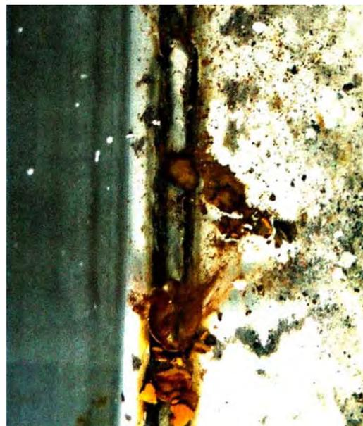
**Figure 6:** This weld within a swimming pool gutter was not cleaned properly and pitting corrosion is occurring along the weld seam. Photo courtesy of TMR Consulting
