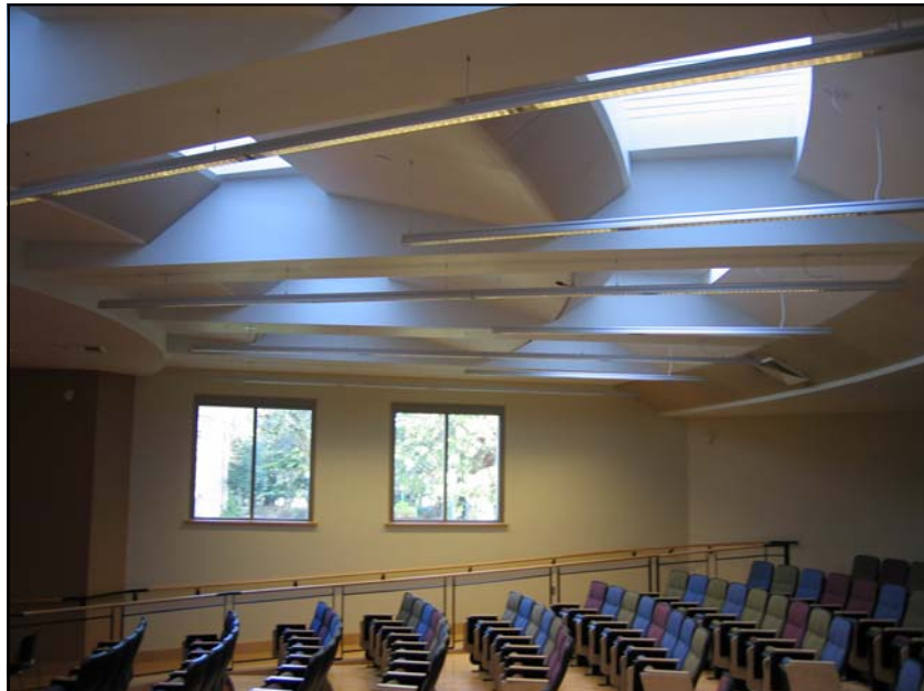
Diffuse top lighting within University of Oregon Lillis Business School lecture halls create a better learning environment.
