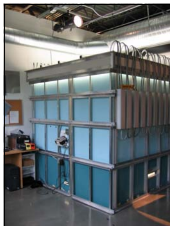
Artificial sky simulator testing a physical model for daylighting potential. University of Washington, Integrated Design Lab
