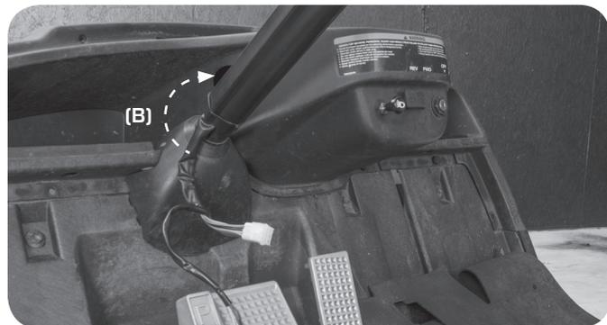
Adjust the Turn Signal position (up or down) to allow Steering Column Cover to fit. Align Wiring inside the raised channel and snap the Steering Column Cover (D) over Steering Column.
