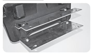
Use the long hardware provided to attach the two Bracket Plates to the Bumper, as pictured below (with stamped "F" facing towards Bumper).
